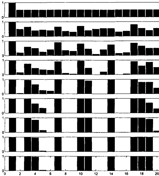
Figure 8.6 The evolution of the CE algorithm for the dodecahedron max-cut problem.
